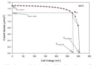
**Figure 6(c).** I-V characteristic under illuminated condition ZnO/ITO thin film annealed at 300°C
