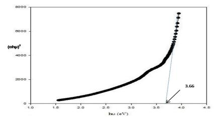
Figure 4(b) Plot of  $(\alpha h\mu)^2$  versus photon energy of ZnO/ITO thin film annealed at 300°C
