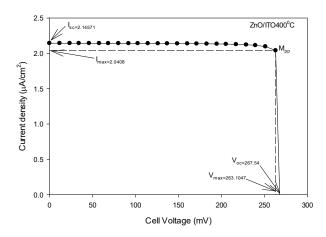
Figure 6(d). I-V characteristic under illuminated condition ZnO/ITO thin film annealed at 400°C
