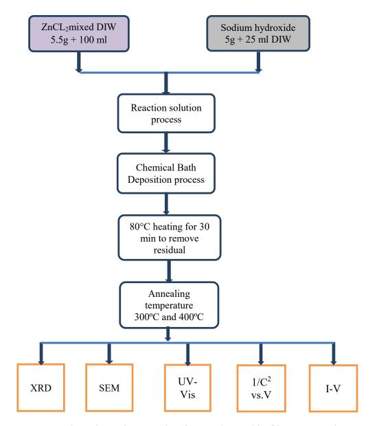
Figure 1. Flow chart of preparation for ZnO/ ITO thin film on ITO glass substrate by using Chemical Bath deposition at various annealing temperature.
