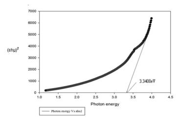
Figure 4(b) Plot of  $(\alpha h\mu)^2$  versus photon energy of ZnO/ITO thin film annealed at 400°C
