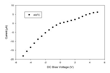
Figure 6(b). I-V characteristic of dark condition ZnO/ITO thin film annealed at 400°C
