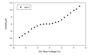
Figure 6(a). I-V characteristic of dark condition ZnO/ITO thin film annealed at 300°C
