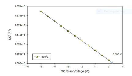
Figure.5(a).1/C<sup>2</sup>vs V characteristic of ZnO/ITO thin film annealed at 300°C
