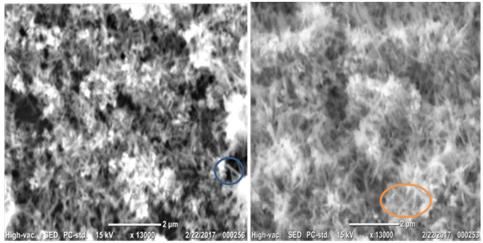
Figure 3(a) and 3(b) showed the SEM photograph of the ZnO/ITO thin film annealed at 300°C and 400°C
